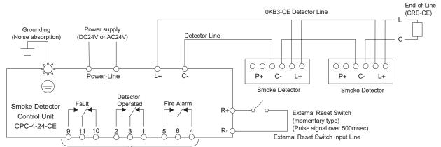
Non-Voltage C Contact: The labels indicate a condition when power is supplied
