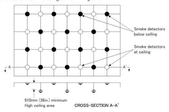
Figure 13: Smoke detector layout accounting for stratification
