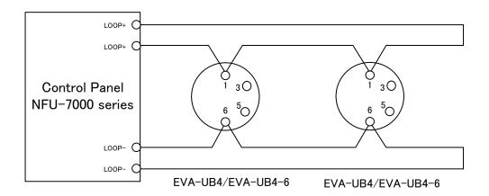
Figure 18: Wiring diagram for EVA-UB4 and EVA-UB4-6
