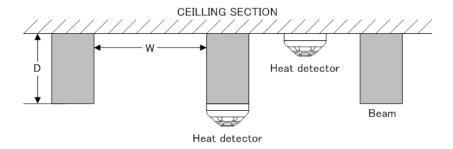
Figure 9: Heat detector spacing — beam construction (side view)
