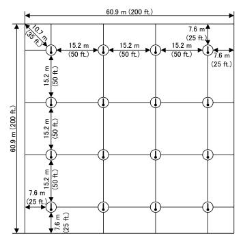
Figure 6: Heat detectors spacing example
