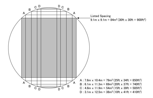
Figure 4: Alternative heat detector coverage configurations
