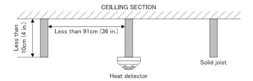
Figure 7: Heat detector spacing — solid joist construction (side view)
