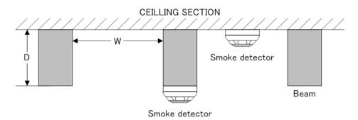
Figure 16: Smoke detector spacing — beam construction (side view)
