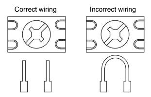
Figure 19: Correct and incorrect wiring method
