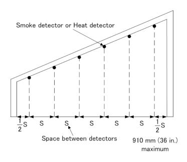
Figure 12: Heat detector spacing — Sloped ceiling (shed type)
