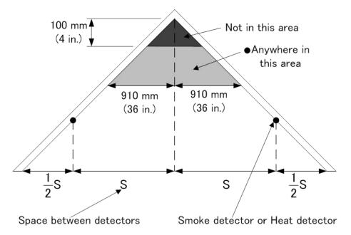
Figure 11: Heat detector spacing — Sloped ceiling (peaked type)
