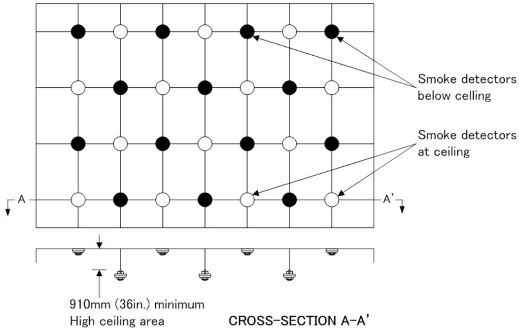
**Figure 2: Smoke detector layout accounting for stratification**
