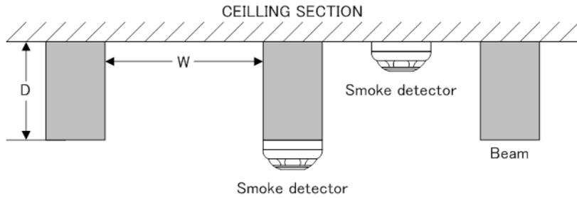
**Figure 5: Smoke detector spacing — beam construction (side view)**
